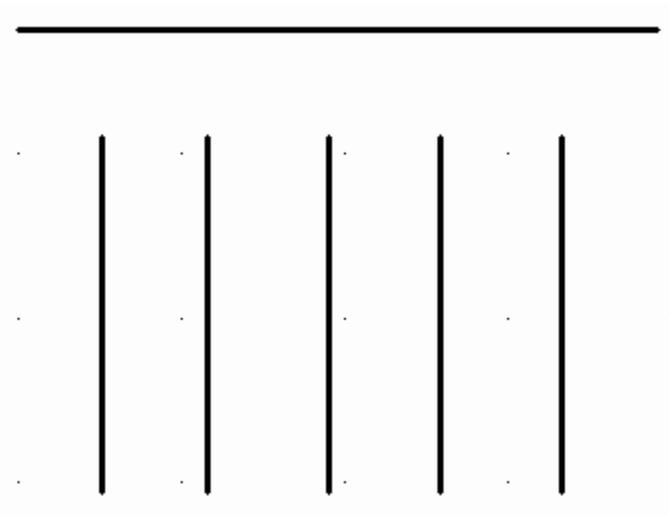
3. **Extend** the vertical lines to intersect with the horizontal (Boundary) Line as shown below.
