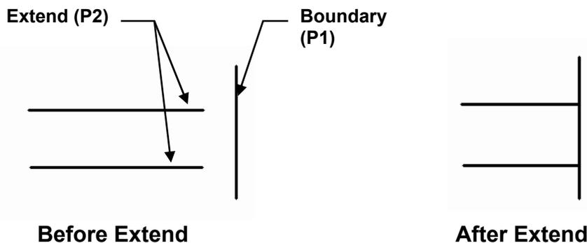
Note: When selecting the object to be extended (P2 and P3 above) click on the end pointing towards the boundary.
